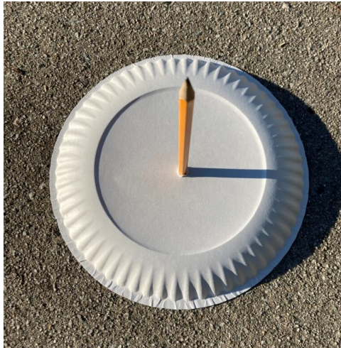
Figure 18: A rudimentary sundial 3 . Empirical hour lines are made by tracing the gnomon shadow at regular time intervals
