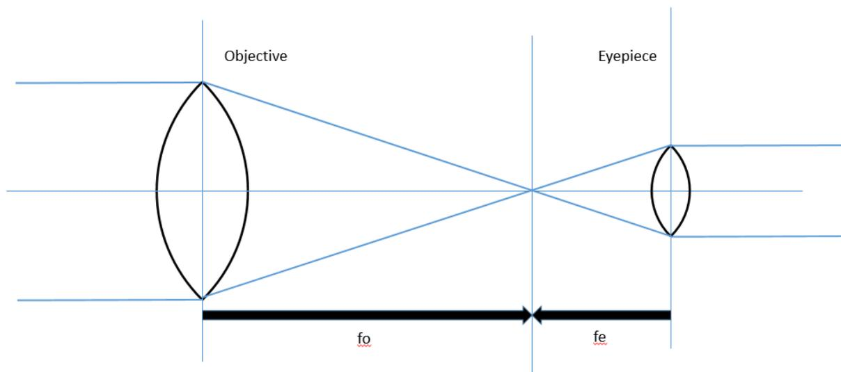
Q10: Assuming light rays from a far away star are travelling parallel to the principal axis, complete the ray diagram above.
