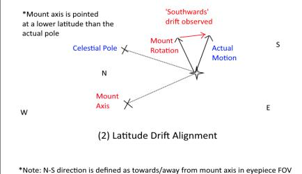
M1 - Discrepancy in mount rotation vs. rotation of celestial pole due to misalignment identified.
